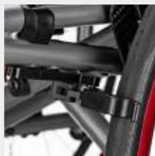
Innovative light brake, swivelling, aluminium
